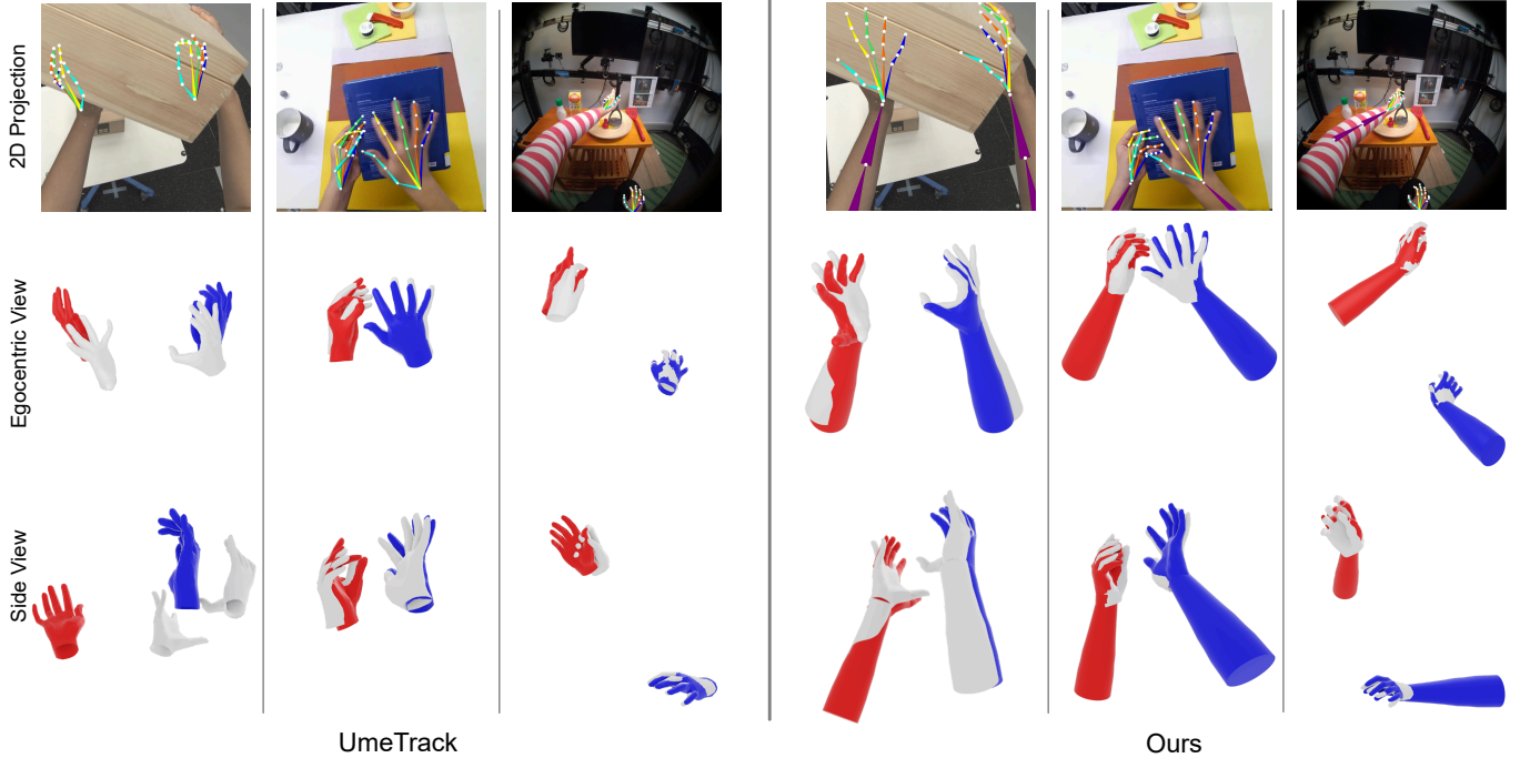
Fig. 19. Qualitative camera-space results on egocentric datasets. We compare our method against UmeTrack [Han et al. 2022] on three datasets with widely different camera intrinsics. Predicted left and right limb meshes are shown in red and blue, respectively, with ground truth highlighted in gray.
